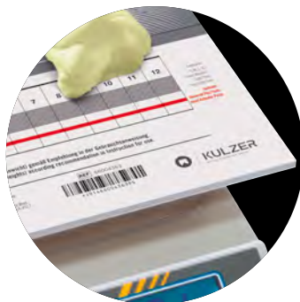
Fig. 37: Always use the scales to ensure exact dosage.
