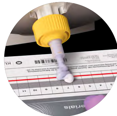
Fig. 34: Discarding of the initial 2–3 cm to adjust the filling levels of the two material components.
