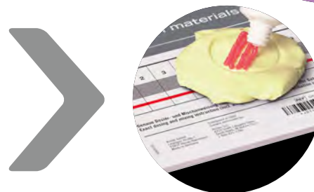
Fig. 41: Removal of the excess material in one go should be avoided as the material can be pushed out from the spoon resulting in underdosing.
