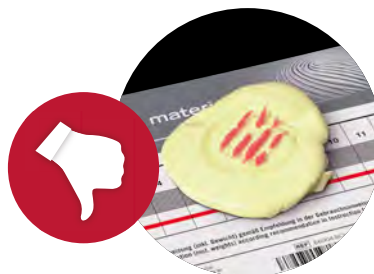
Fig. 46 – 48: Correctly dosed strands (left). In comparison, unevenly and too thin (middle) respectively too thick dispensed strands (right).
