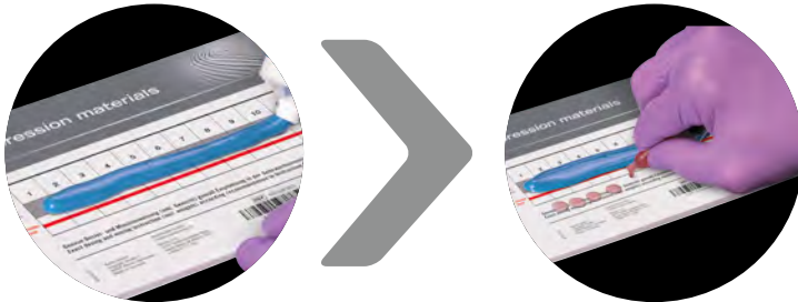
Fig. 54 & 55: Pre-dosing of base materials and liquid activator.
