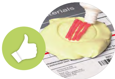
Fig. 46 – 48: Correctly dosed strands (left). In comparison, unevenly and too thin (middle) respectively too thick dispensed strands (right).
