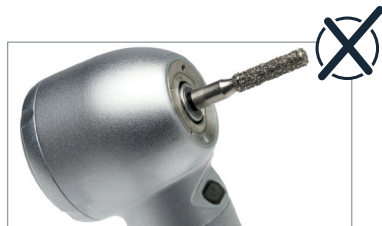
Groove in the area of the guide bushing - no longer visible
