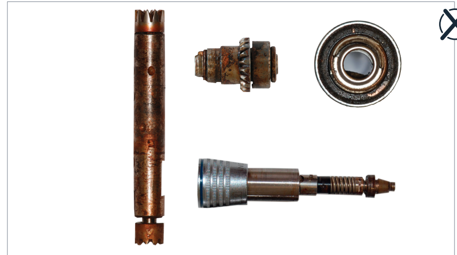
Improperly serviced handpieces
