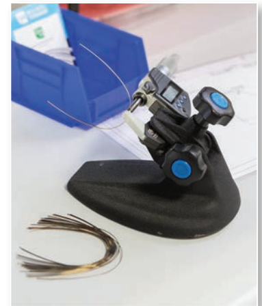
The diameter of all wires is tested for consistency of size.
