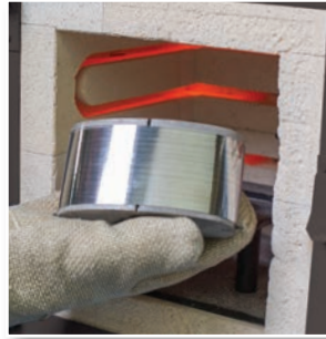
Heat-treatment sets the archform shape to wire.
