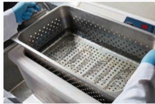
An ultrasonic, aqueous clean bath removes all soils and contaminants from wire.
