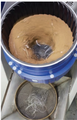
Wires are mechanically polished in a proprietary media with an abrasive polishing agent ensuring the best wire surface for optimal sliding mechanics during clinical treatment.
