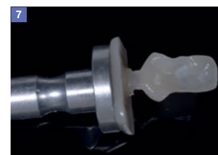
Machining of the NUMERYYS HC A2/12 block
