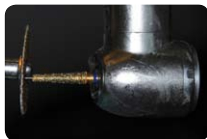
Fig. 6: Adjustment of the guiding pin with a sandpaper disk.
